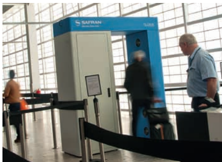
Pic 3: Explosive detections systems based on QCL technology have been successfully trialled at Glasgow airport in the UK Credit: Cascade Technologies
