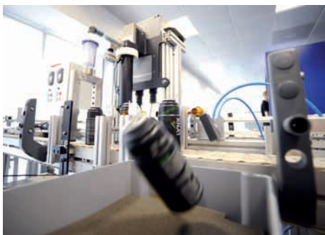
Pic 2: An aerosol can is rejected from the high-speed production line after a QCL-based spectroscopy system detected a leak Credit: Cascade Technologies
