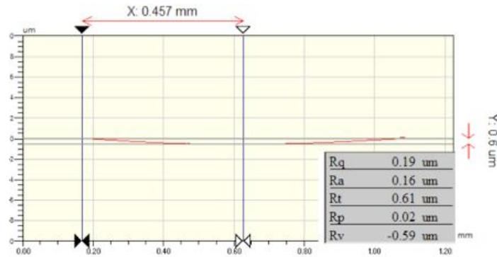
Figure 8. Surface topography of metallized mirror segment
