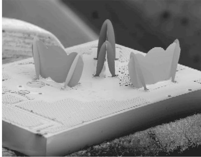
Figure 1. SEM micrograph of Michelson interferometer
