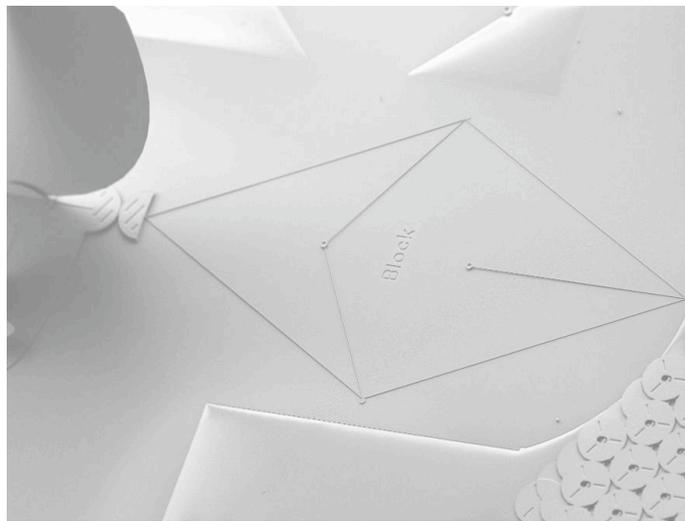
Figure 6. SEM micrograph of Straight-Line-Generator (Peaucellier linkage)
