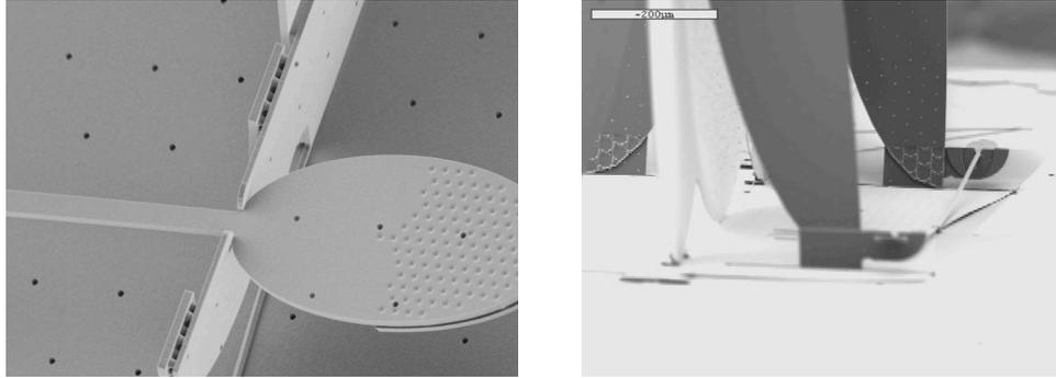
Figure 5. SEM micrograph of locking features
