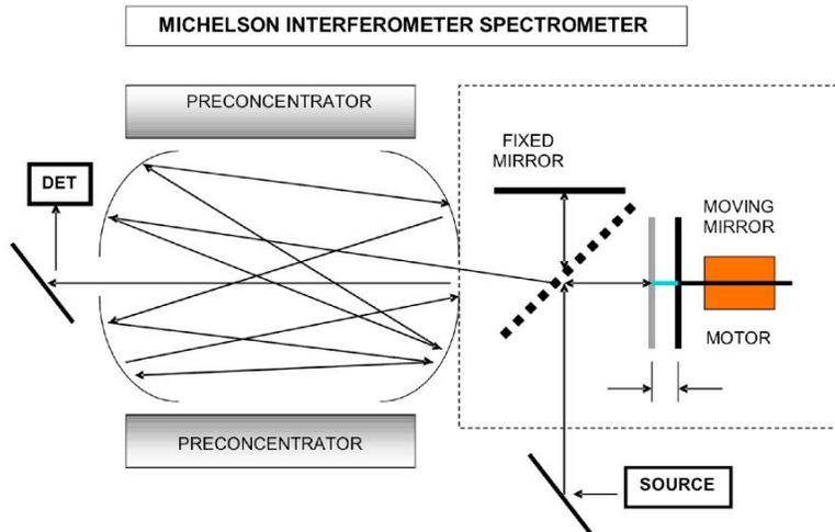
Figure 2. Schematic diagram of FTIR operating principle
