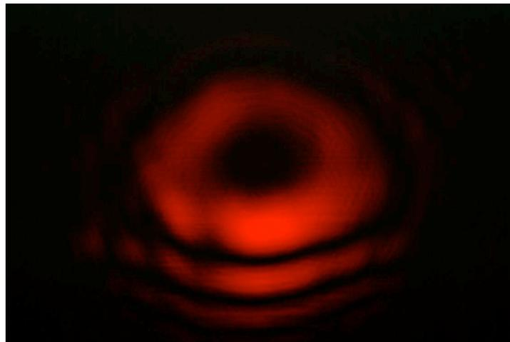
Figure 9. Acquired static Interferogram from Block MEMS Michelson interferometer in zero path difference at 0.6328 $\mu\text{m}$
