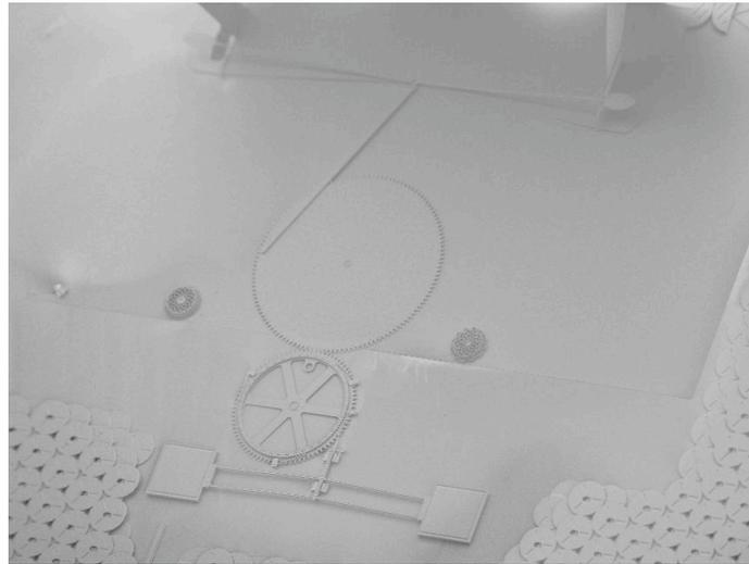
Figure 7. SEM micrograph of actuator and gear system
