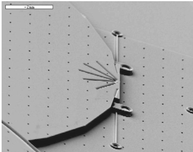
Figure 4. SEM micrograph of flexure hinges and staple retainers
