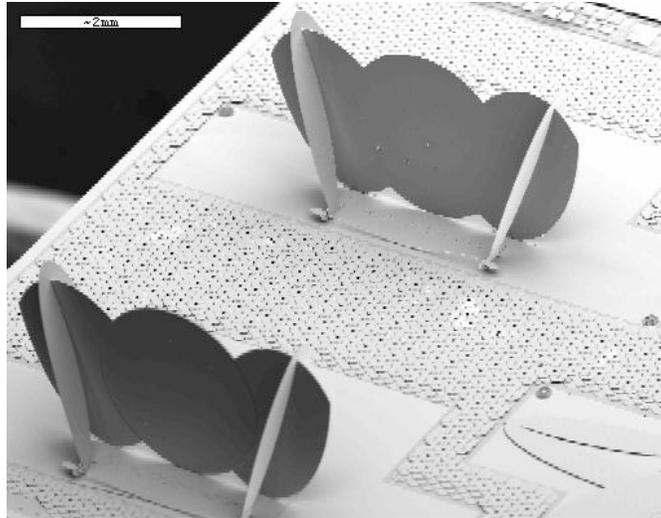
Figure 3. SEM micrograph of assembled, individual mirror segments
