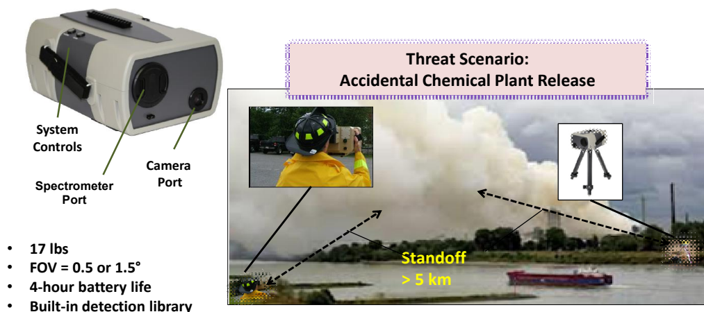
Figure 3: PORTHOS is a passive detection system that incorporates a FTIR spectrometer with detection algorithms and a low-light camera.
